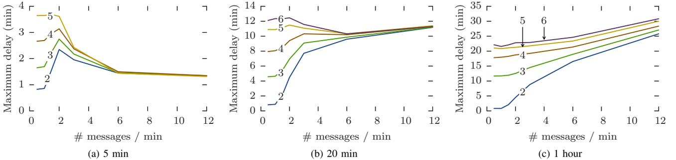
Fig. 7. Average maximum delivery delay vs message creation rate for different message lifetimes. (1) local-only UHF, (2) Immediate, (3) Early, (4) Midtime, (5) Late, (6) Last moment
