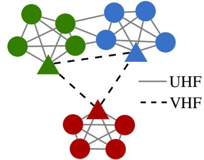
Fig. 1. Hybrid deployment of VHF/UHF radios. All nodes are equipped with UHF radios. Leaders, depicted by triangles, also have a VHF radio.
